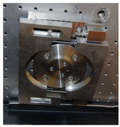
Mounting clamp hanging under AO system ready to accept instrument
