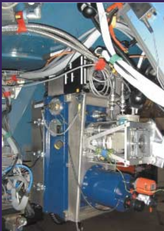
Rear view of UFTI mounted on UKIRT The instrument is suspended from the mirror cell. Light enters the cryostat at the bottom left and is collimated by a diamond-turned aluminium mirror located in the blue tube at lower right. The closed-cycle cooling system is contained in the aluminium trusses at middle right. The instrument and mounting frame weighs about 140 kilograms
