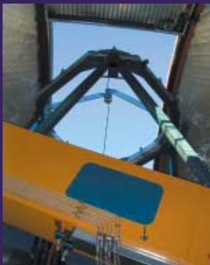
A view of the UKIRT telescope top-end, showing the new secondary mirror and support structure, and the dome aperture
