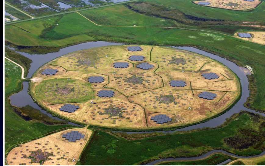
Fig. 1. Aerial photograph of the Superterp, the heart of the LOFAR core, from August 2011. The large circular island encompasses the six core stations that make up the Superterp. Three additional LOFAR core stations are visible in the upper right and lower left of the image. Each of these core stations includes a field of 96 low-band antennas and two sub-stations of 24 high-band antenna tiles each.
