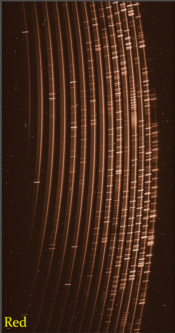
Raw X-shooter spectrum of a Quasar. The wavelength increases from bottom to top of each spectrum, and from left to right. The spectrum of the quasar is the thin bright lines visible in each of the orders. The short bright nearly horizontal lines are atmospheric airglow lines while the thermal emission increases sharply above 2um in the right hand spectrum
