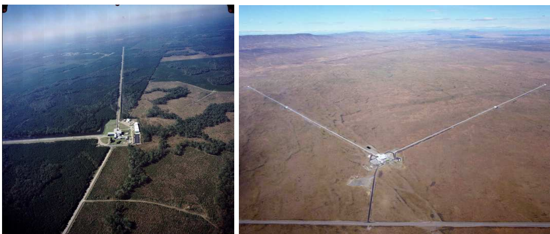
Figure 5: Photos of the two aLIGO detectors in Livingston (Louisiana, left) and Hanford (Washington, right). These are Michelson interferometers, where each arm has a length of 4 km. The two detectors are located 3,000 km apart to allow the distinction of an astronomical event from local noise sources (source: LIGO website).
